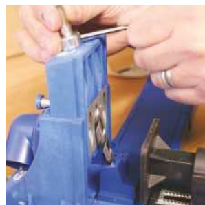
▲ Once the guide block is at the right height, the drill can be set up with the stop collar
